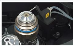
Dual micro nozzle geometry automatically keeps the proper amount of water on the tip of water immersion objectives.
