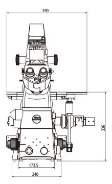
Single layer configuration with an Epi-FL module
