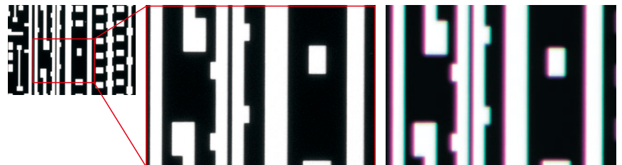
Apochromat optics (captured with SMZ1270+Plan Apo 1x/WF)
